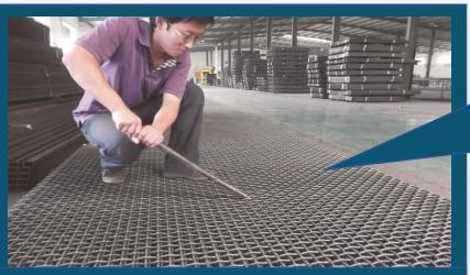
Good Quality woven mesh has zero tolerance to any movement within crimp or weave.
